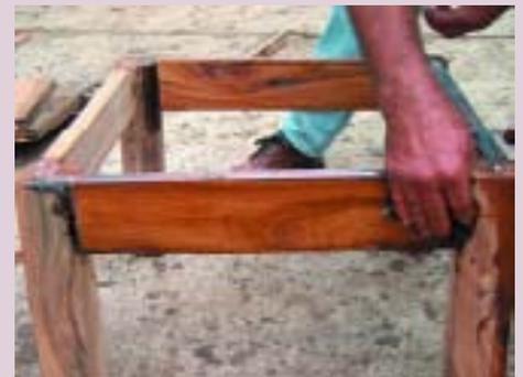
**Move onto the legs and the frame, coating as before.**
