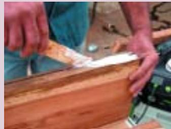
**Cut feather out of 3mm plywood and spread glue onto the edges of the planks.**
