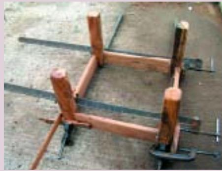
**The legs and frame of the coffee table, glued and clamped.**
