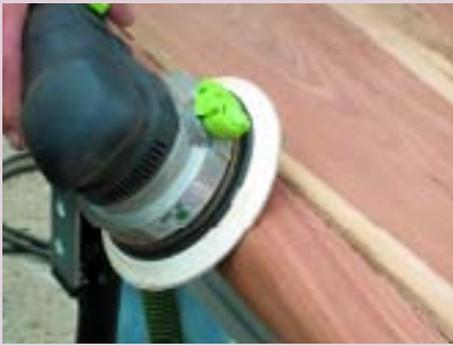
**When all unsightly scratches are removed, use an orbital sander with 150 grit paper to polish the top.**
