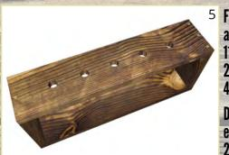
From one side, measure and make marks at 114.5mm, 207mm, 299.5mm, 392mm, and 484.5mm.
