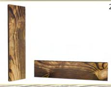
2 Cut two pieces measuring 600mm x 144mm for the top and bottom.
