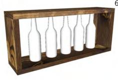
Insert the clean glass bottles in the holes in the top.
