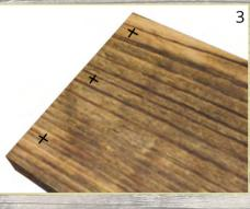
3 Use 3.5mm x 40mm Eureka Cut screws to construct the box.
