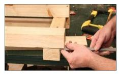
**8.** Measure out the back rest so that it sticks over the same length both sides of the bench.
