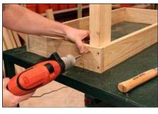
**3.** Finish driving all the Decking screws in on the sides and on the front of the frame
