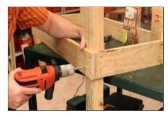
**6.** Drive 2 decking screws through the frame into the back legs on either side.
