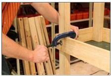
**5.** Secure the back feet with a clamp to hold it in place.
