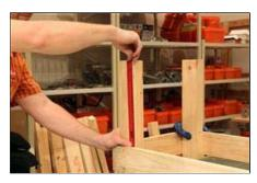
**4.** Measure out the back feet so that the bench will stand flush on the ground.
