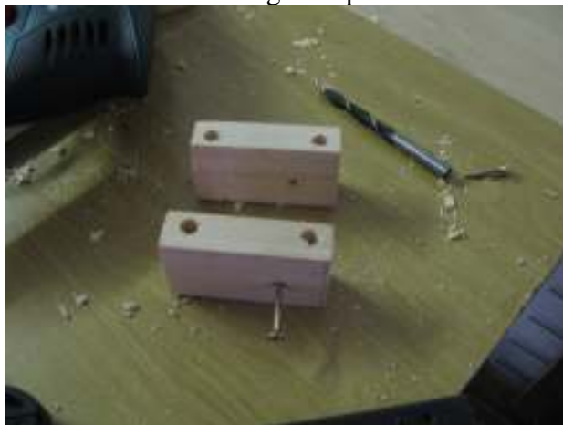
Item 4.9: 4.5mm holes drilled
