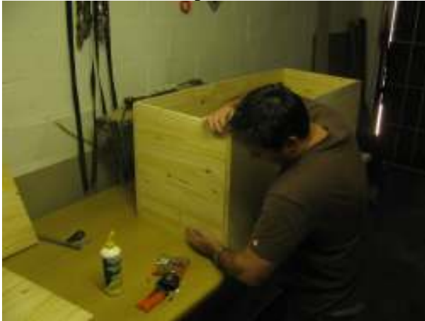
1.8 Position second 1200mm length and screw in screws
