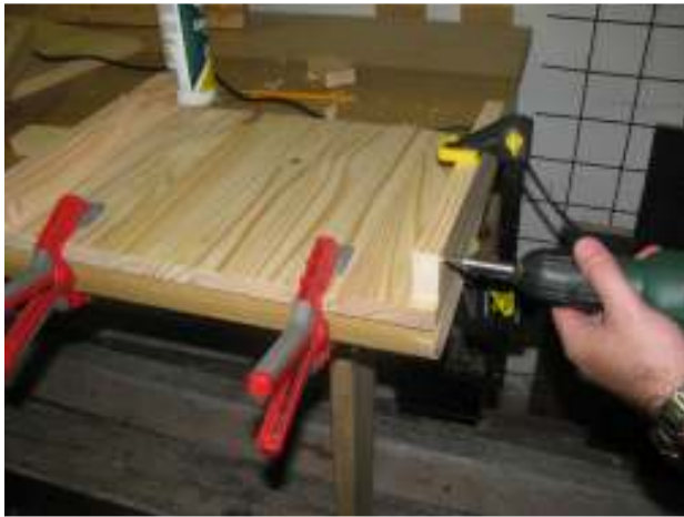
Item 4.7 Drilling of pilot hole
