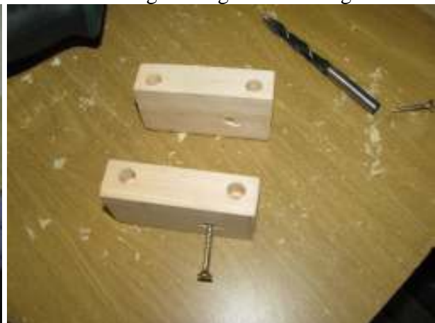
Item 4.9: 9mm sink holes drilled
