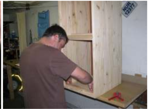
Item 3.5 Fitting battens onto short sides
