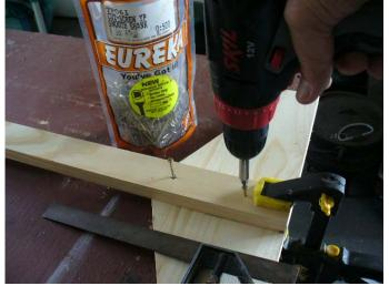
4.2 Glue and screw the bottom and middle horizontals in place. The 2 bottom ones go right at the bottom about 25mm from the "toes" of the feet. The next 2 go in the corners against the uprights and the feet, in line with, or slightly below the top of the downwards line of the feet.
