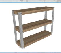
On one side of the aluminium, drill 3.5mm holes in the centre & 15mm in from each end. On the adjacent side, offset the holes so that the screws don't bump into each other when screwed in.
