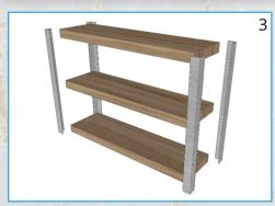
This is how the various components of the shelf go together. Distance between the shelves is 239mm.
