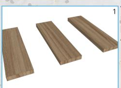
The shelves, each 800mm long, are cut from shop bought 220mm wide x 44mm thick planks.
