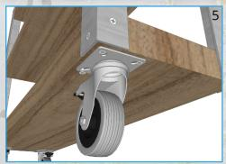
5 Secure the castors to the four corners of the underside of the bottom shelf.
