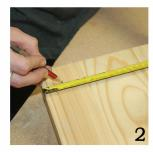
2. Measure 30mm in from each side to determine where to drill the holes for the threaded rod.
